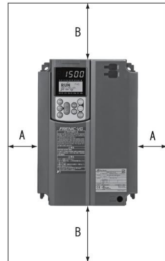
Figure 2.1-1 Mounting Direction and Required Clearances
