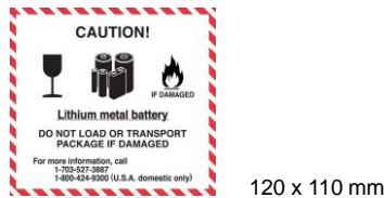
Figure 7.4-4 Label to be Attached to Outer Wrapping
