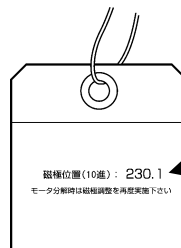
Figure 4.4-2 Magnetic Pole Position Offset Labels
