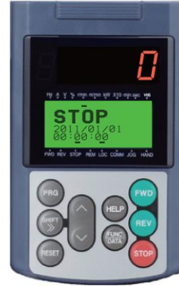
Figure 4.2-1 Display of the LED Monitor at Power-on
