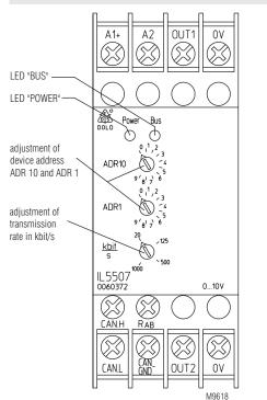
The configuration is made with the programming software PN 5501 in conjunction with minimaster IL 5504 / IN 5504 or e.g. with ProCANopen. The corresponding configuration file on CD can be ordered under order no. PN 5501, article no. 0052860
