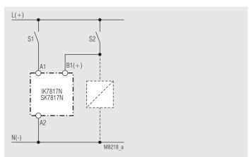
Control with parallel connected load
