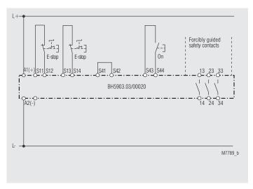
$BH\,5903.03/00020$  with two E-Stop loops (single-channel), automatic restart after phase failure and manual restart after E-stop.
