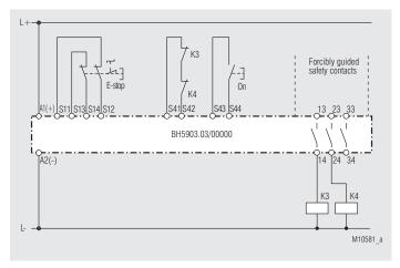
BH 5903 with external contact reinforcement
