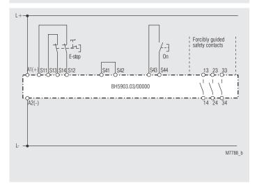
BH 5903.03/00000 with one E-Stop loop (2-channel), automatic restart after phase failure and manual restart after E-stop. Automatic reset ist only active when no E-Stop was operated before phase failure.
