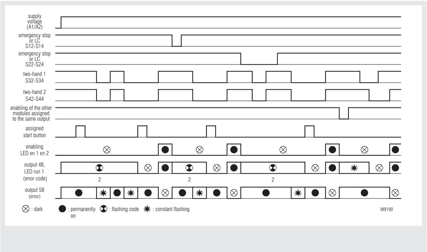
Emergency stop and / or light curtains, manual start, 1 two-hand control type IIIC; functions: 6, 7 or 8
