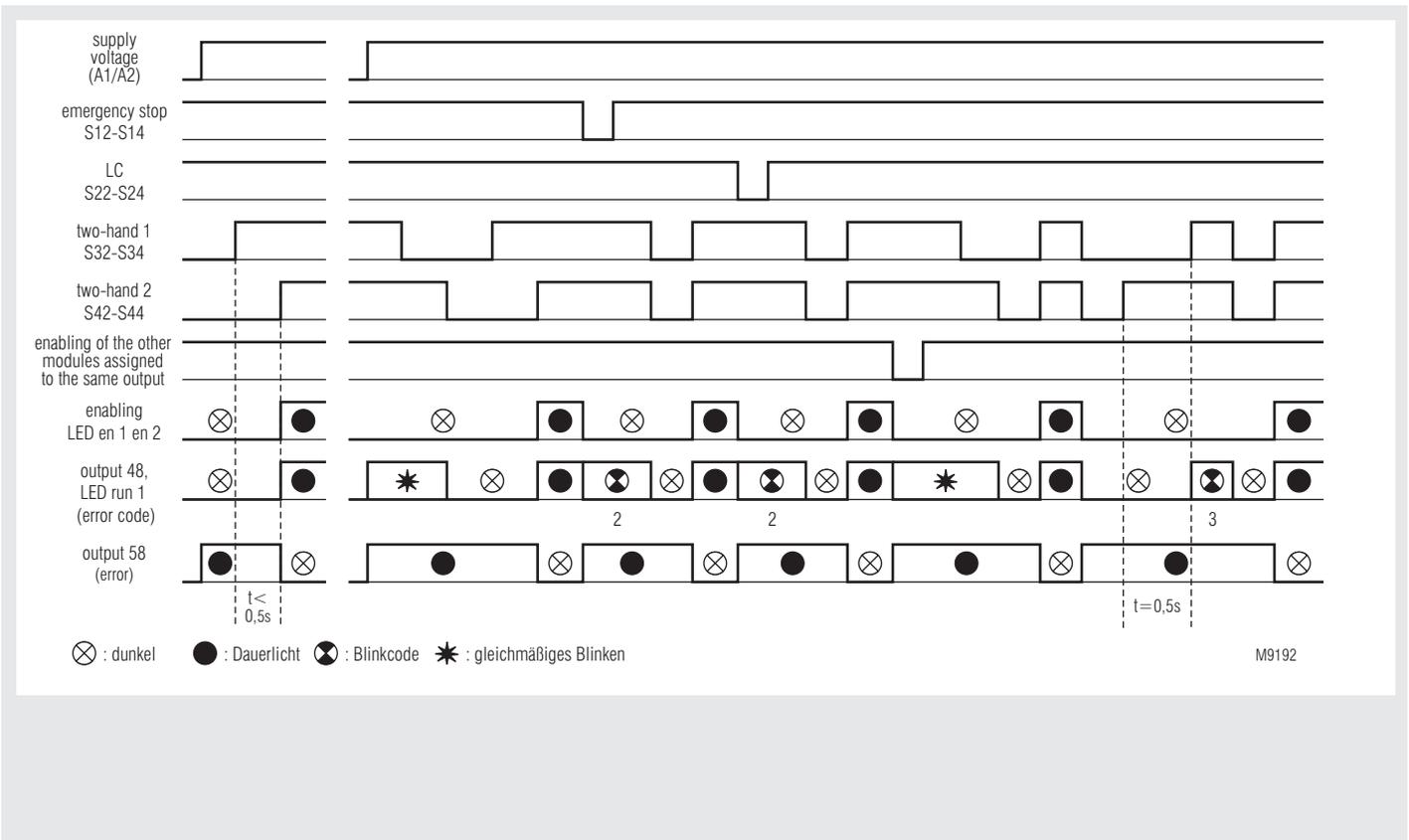
1 Emergency stop and 1 light curtain, Autostart, 1 two-hand control type IIIC; function: 9
